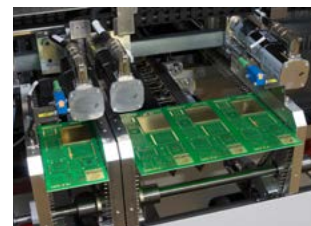
Multi-track conveyor for variable PCB widths
