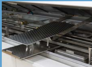
Retractable nozzle sheets for quick maintenance
